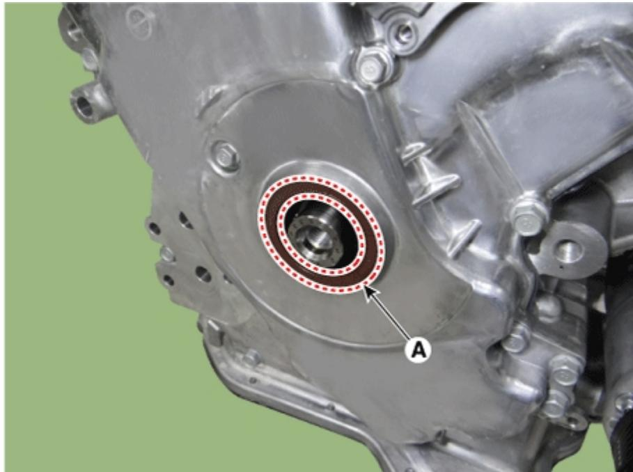
3. Using SST (09231-3C100), install a new front oil seal.
